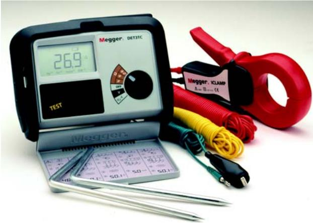
The testing of earth systems has relied for many years on the tried and tested “Fall of Potential” and other related methods. These methods give reliable results, but can be time consuming. To measure an individual electrode’s earth resistance requires the disconnection of the electrode being tested from
